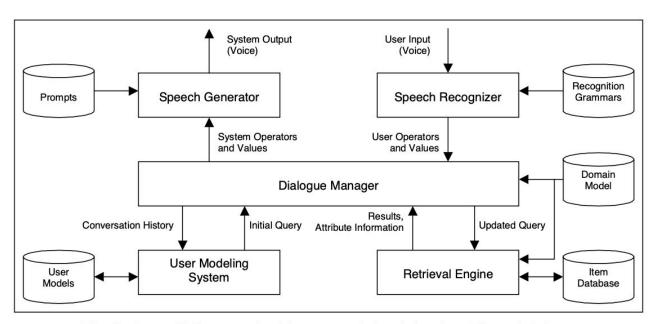
Fig.1: Overall System Architecture of the Adaptive Place Advisor.
